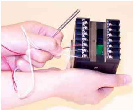
Pic: 3-wire RTD connection
